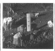
pedestals seldom survive the winter due to frost heave and freezing and thawing). The rock wasn't necessarily on the soil surface at the beginning of the season. Thus the pedestal may record less than the actual amount of erosion.
