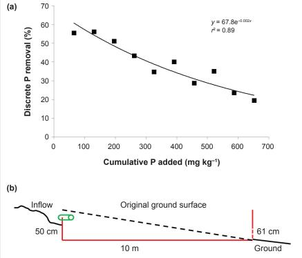
words, it takes 30 seconds for the solution to pass through the PSM. The P sorption is initially very high, but with further P loading, the PSM is not able to sorb as much P as it did previously. The shape of the curve varies between PSMs, retention times, and inflow P concentrations. A detailed discussion of design curves is provided by Stoner et al. (2012).
