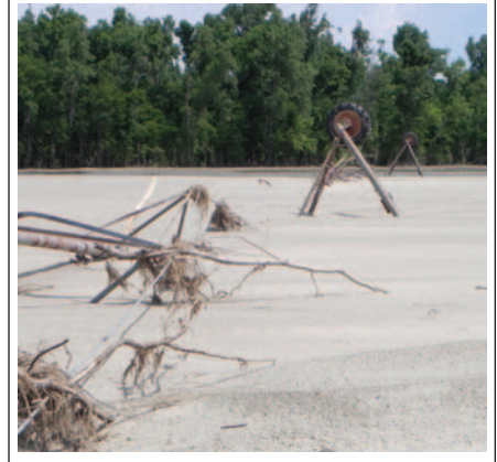
Figure 4 An irrigation system was overturned by the force of floodwater and wind and then buried by thick sand deposit. Photo courtesy of Brett Miller, Soil Conservation Technician, USDA Natural Resources Conservation Service.
