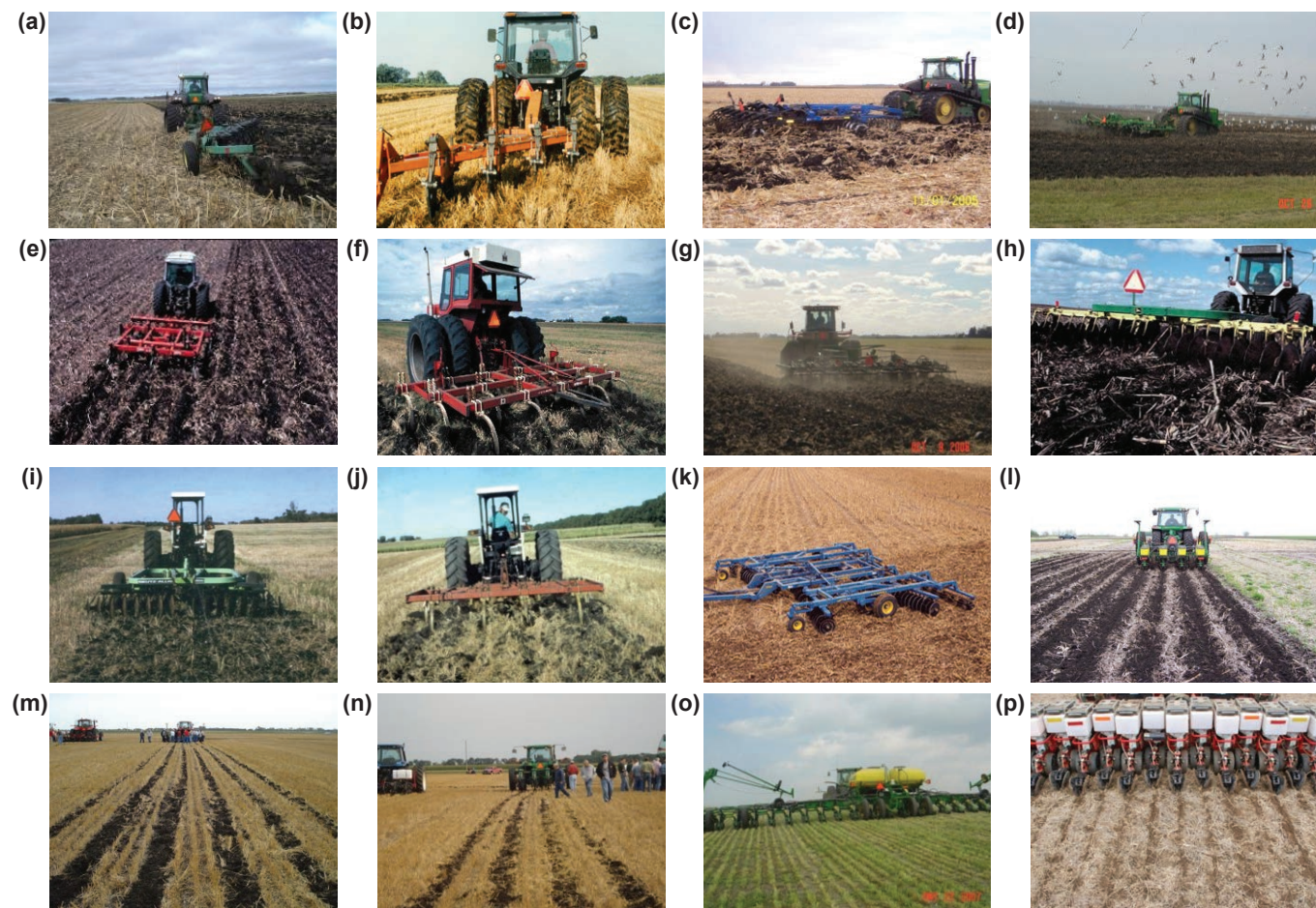
Collection of several different types of “conservation tillage” tools and planters illustrating a wide range of tillage depths and degrees of residue incorporation (from left to right and top to bottom): (a) conventional inversion moldboard plow, (b) paraplow, (c) deep ripper combination tool, (d) deep field cultivator combination tool, (e) field cultivator tool rigid tine (photo courtesy of the Natural Resources Conservation Service [NRCS]), (f) deep field cultivator spring tine (photo courtesy of NRCS), (g) deep field cultivator rigid tine, (h) heavy-duty disk harrow (photo courtesy of NRCS), (i) shallow field cultivator spring tine, (k) vertical tillage tool (photo courtesy of NRCS), (l) high disturbance strip tillage implement combination tool, (m) strip/zone tillage implement in wheat stubble, (n) strip tillage implement combination tool rigid tine, (o) disc opener no-till planter into alfalfa stubble, and (p) disc opener no-till planter into dead residue (photo courtesy of Dave Brandt).
