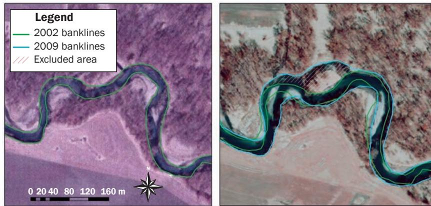
gons would represent the channel elevation. Therefore, using data found adjacent to (outside of) each of these polygons, we estimated the surface elevation of the erosional polygon prior to the erosional event. The erosional polygons were buffered outward by 5 m (16.4 ft), creating a “ring” around each. Note this 5 m outward buffer thereby went 3 m (9.8 ft) beyond the originally digitized polygon to include areas just above the bank on one side of each erosional polygon.
